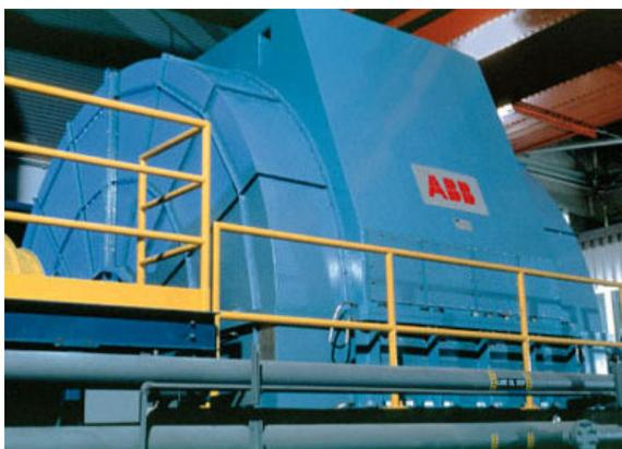
*New 100-MW (135,000-HP) synchronous motor used to operate the NTF wind tunnel*
